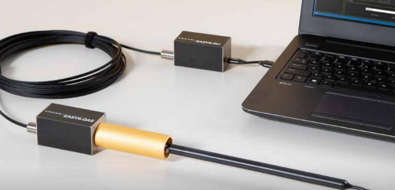
widely used Electromagnetic (EM) Exposure Acquisition System EASY4/MRI. It is smaller, more cost-efficient, and directly connects our classic specific absorption rate (SAR), temperature and field probes via an optical link (EASY6-DAE + EASY6-RU) to the computer. The user-friendly EASY6 software allows the acquisition of data from 1-10 probes while
