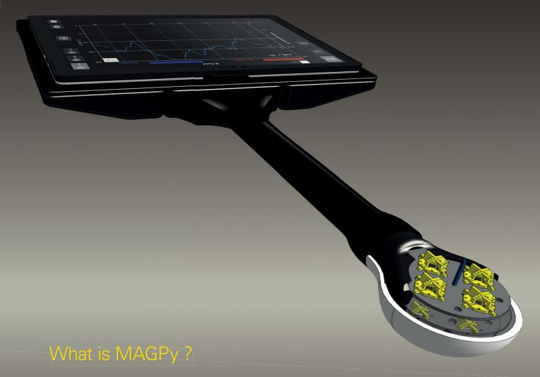
Probe System (MAGPy) is a cutting-edge all-in-one instrument for fast and reliable testing of compliance with basic restrictions (BR) and reference levels (RL) from 3 kHz to 10 MHz. It greatly reduces the exposure over-estimation for wireless power transfer (WPT) systems and any other near-field sources. The device comprises 24 small time-domain loop sensors arranged at the corners of a cube, for determining the
