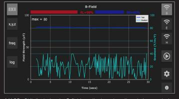
MAGPy GUI displaying the B-field amplitude and gradient during a typical measurement. Compliance with both reference levels and basic restrictions are shown as exposure ratios, and are continuously updated during the measurement.
