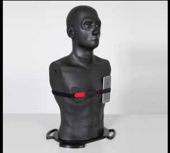
POPEYE10 upper body including HEAD, CHEST, and ABDOMEN phantoms with anatomical EYES and EARS
