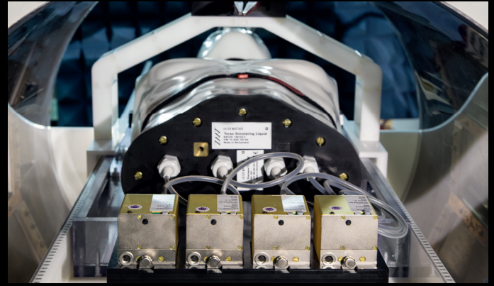
MRI-safety evaluation suite: Torso phantom and EASY4MRI
