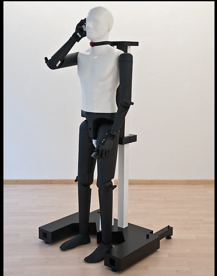
POsable Phantom for Electromagnetic sYstems Evaluations (POPEYE V5.x)
