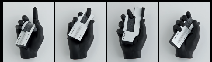
SHO hand phantoms with CTIA-compliant handgrips
