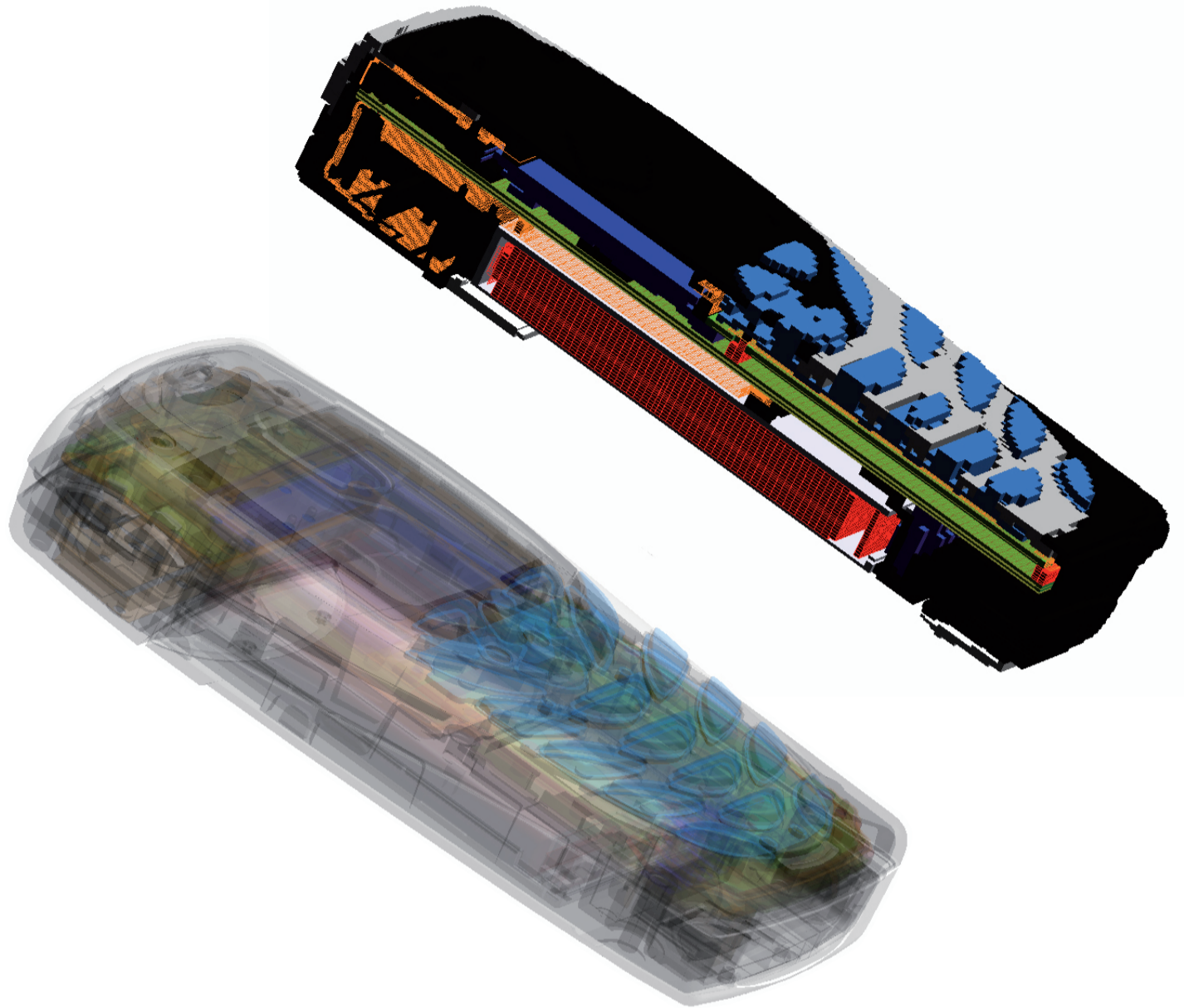
Figure 3: CAD model and discretized model of the NOKIA 8310: The mesh is truncated by 8 layers of UPML media leading to an overall mesh size of 5.6 million voxels whose size varies between 0.01 mm and 12 mm. The default time step is 32CFL.
