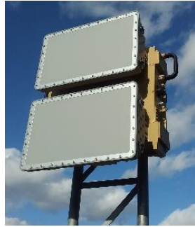
Figure 3: Two 5° beam-width antennas deployed on radar.
