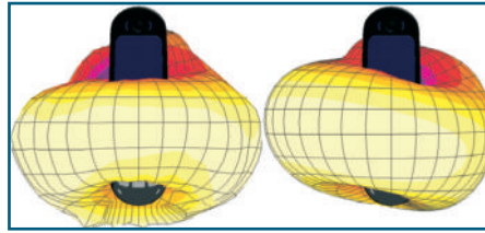
Figure 5: Simulated (right) and measured (left) radiation pattern of the V180 phone: 3D freespace comparison.
