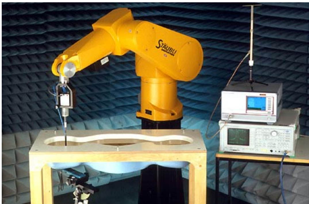
Figure 5.2, The measurement arrangements with DASY3 from SPEAG's homepage
