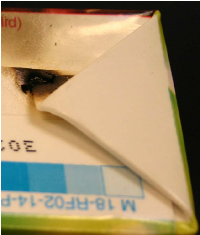
Figure D.1. An ordinary carton where ionization has left burn marks.
