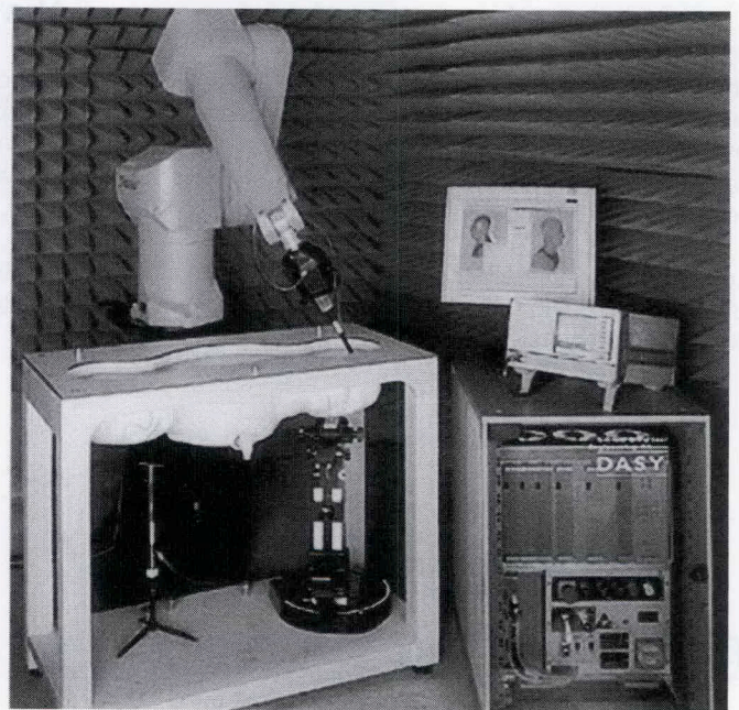
Figure 2. The automated dosimetric assessment system, DASY4: measurement of a mobile phone.
