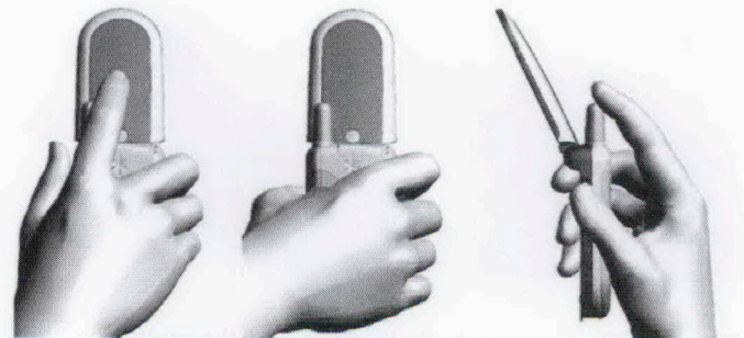
Figure 6. The CAD representations of the hands for the simulations: H1 (left), H2 (middle), and H3 (right).
