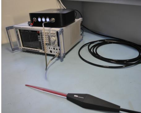
After the pin is inserted the *Remote Unit* signals standby mode by "breathing" of the LEDs on the front. The *Remote Unit* is ready for use now.
