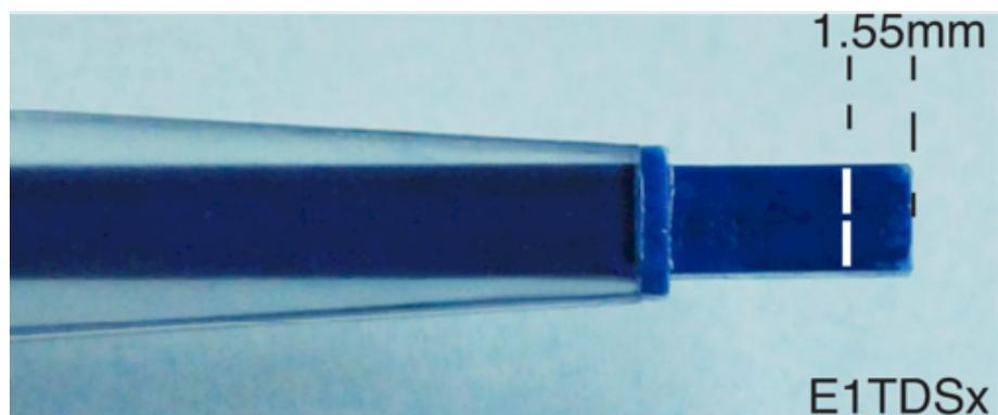
The dipoles of the E1TDS sensors are centred in the *TDS* probe tip centre. The tip to dipole centre distance is in both case 1.55 mm.
