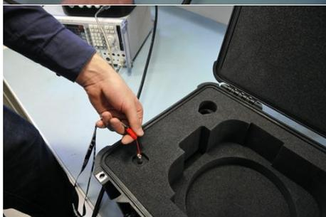
Insert the activation pin on the front left of the *TDS Remote Unit*.
