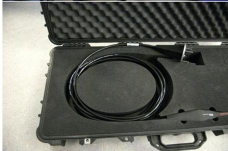
Coil up the fibre optical patch-cord in 7 relatively loose turns in the foam cutout as shown on the left.
