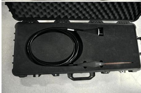
Insert the connector handle in the foam cutout. If the length does not fit you may either use one of the secondary cutouts or re-adjust the coil radius of the fibre optical patch-cord.
