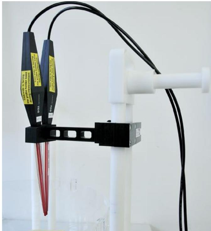
The holder consist of two separate parts. The first one is attached directly to the legs of the Dual Cylinder plantom. The second one is snapped to the first one with a simple click mechanism and holds the probes, both during calibration and measurement.
