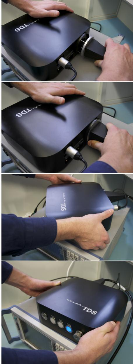
4) Once the rotation is completed, the cable connector can be fully inserted into the shutter mating the cable's MU8 connector with the MU8 connector inside the shutter. **Please make sure that the cable connector is inserted straight (fully orthogonal) into the *Remote Unit* housing)**
