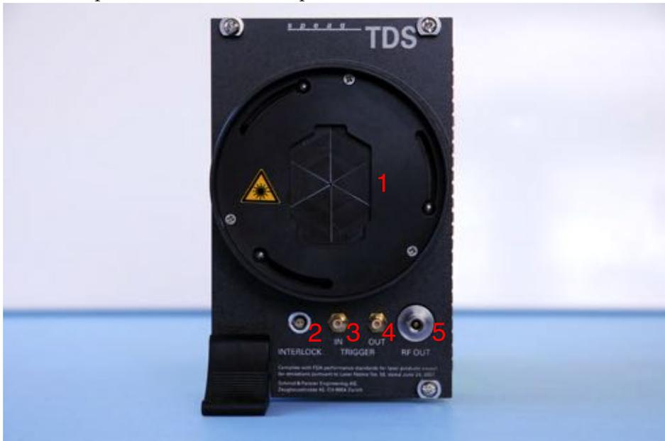
1. Shutter with MU8 fibre optical connector
