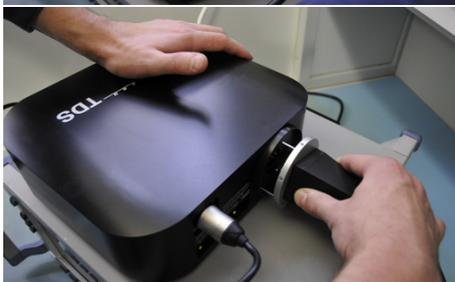
Once the *Remote Unit* is powered all three LEDs will start flashing indicating a "Link Error" as no probe is connected yet.
