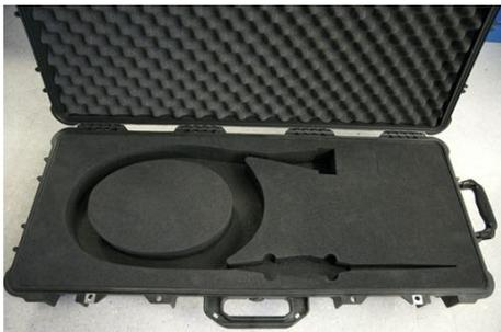
Prepare and open the *TDS* probe transport case. It is recommended to not yet disconnect the probe from the remote unit to protect the fibre optical connector during packing.
