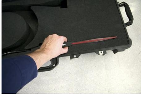
Insert the probe into the foam cutout as shown on the left. Make sure the probe is fully inserted in the foam.
