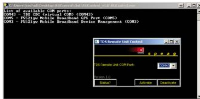
Pressing the Activate and Deactivate buttons is switching on and off the *TDS* sensor. Upon the first activation of the sensor the type and serial
