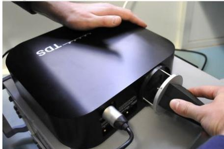
Disconnect the probe from the *TDS Remote Unit*.
