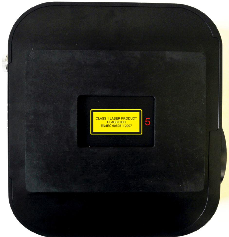
Figure 1: Standalone *TDS Remote Unit* safety marking
