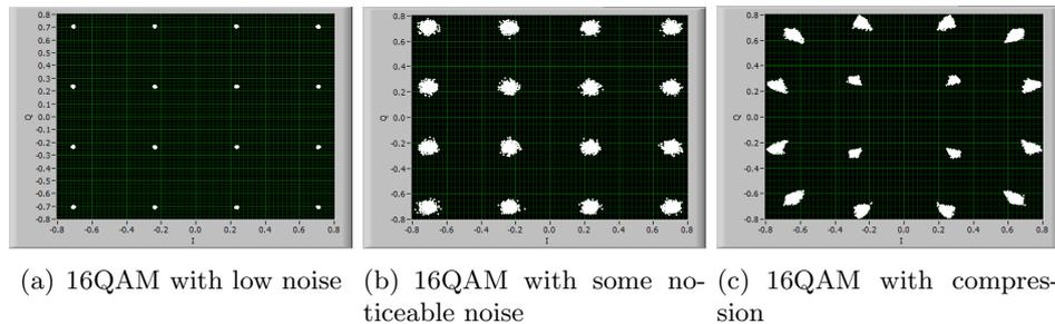
Figure 6.8: Real-life measurement data showing AWGN noise and compression in the transmission channel
