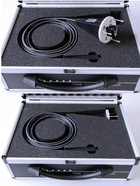
Coil up the fibre optical patch-cord in few relatively loose turns in the foam cutout as shown on the left.
