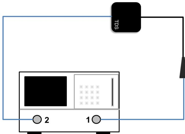
Figure 6.11: AM-AM and AM-PM test setup using a 2-port VNA. The remote unit of the *RFoF1P* system is connected to port 2 using a coaxial cable (in blue). The *RFoF1P* transducer is attached to port 1 using another coaxial cable.
