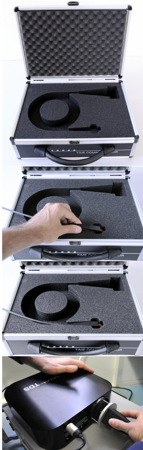
Prepare and open the *RFoF1P* probe transport case. It is recommended to not yet disconnect the probe from the remote unit to protect the fibre optical connector during packing.
