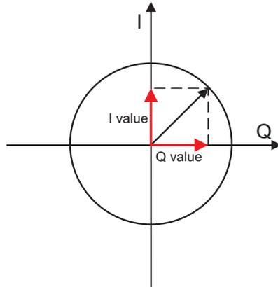
Figure 6.2: The resulting signal is represented as a vector sum of the in-phase (I) and quadrature (Q) components
