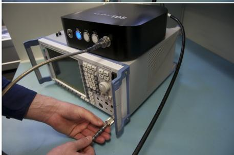
Connect the male end of the PC 3.5 mm cable to the RF in connector of your measurement receiver. (Use torque wrench for reliable mating.)
