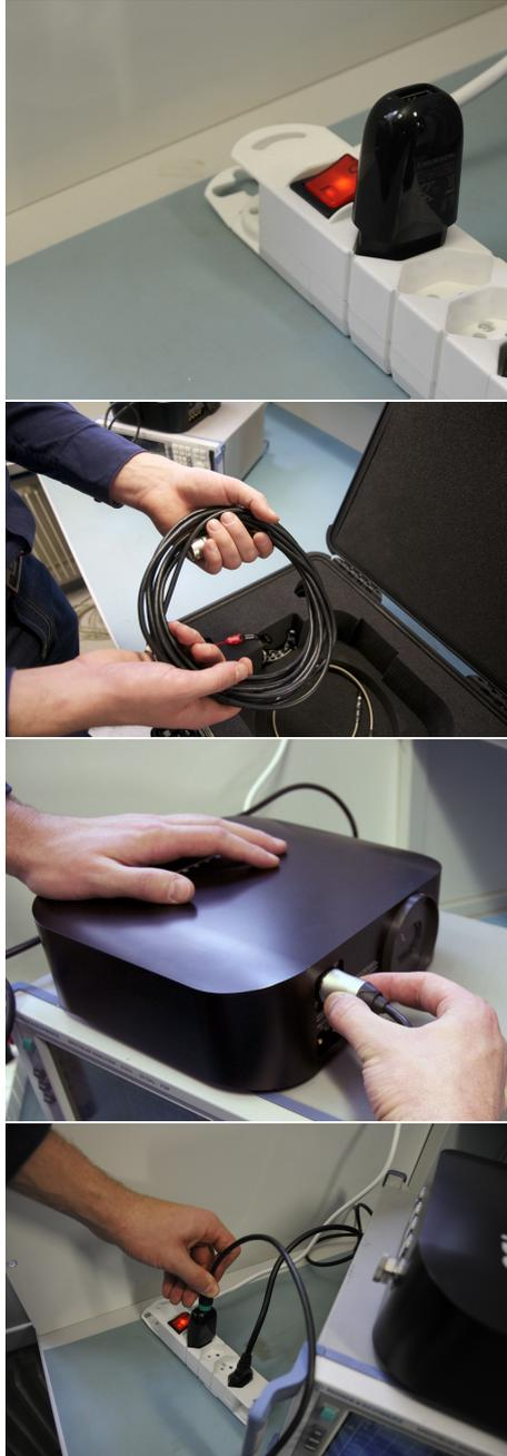
Place the USB power supply inside a power outlet socket. Connect the *Remote Unit* to the USB power supply using the included USB cable. Connect the USB cable with the Type B connector to the rear side of the *TDS Remote Unit*. The delivered cable provides an industrial grade USB connector (Neutrik), which has an automatic locking mechanism. To release the Type B USB connector, pull the metallic sleeve around the connector backwards to release the locking mechanism and then remove the cable.
