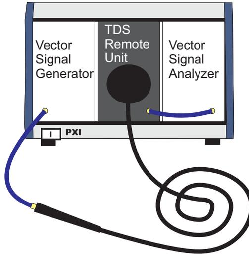
Figure 6.7: Simplified diagram of the setup used for the modulation analysis of *RFoF1P*. The signal generator provides a modulated signal at its output. This is transported using *RFoF1P* and delivered at the RF input of a vector signal analyzer. An external computer is used for control and visualization of the results.
