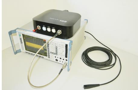
After the pin is inserted the *Remote Unit* signals standby mode by "breathing" of the LEDs on the front. The *Remote Unit* is ready for use now.
