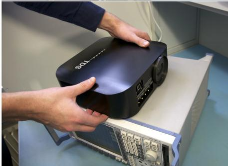
In a typical setup the *TDS Remote Unit* is placed close to the measurements receiver, e.g., on top of a spectrum analyser as shown on the right. **Note: The *TDS* remote unit contains magnetic components and should not be brought close to strong static magnetic fields such as a Magnetic Resonance Imaging system.**
