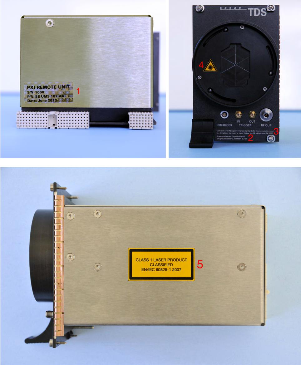
Figure 2: PXI TDS Remote Unit safety marking
