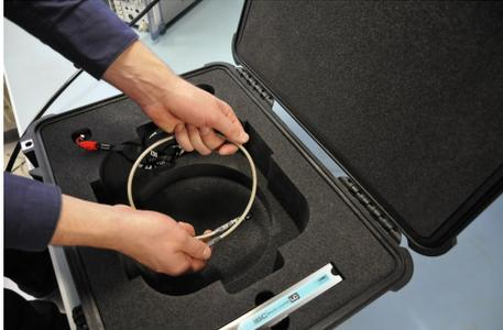
Use the PC 3.5 mm cable delivered with the *TDS Remote Unit* and connect the female end to the 3.5 mm NMD connector at the front of the *Remote Unit*. To fasten the NMD connector turn the large nut counter-clockwise.
