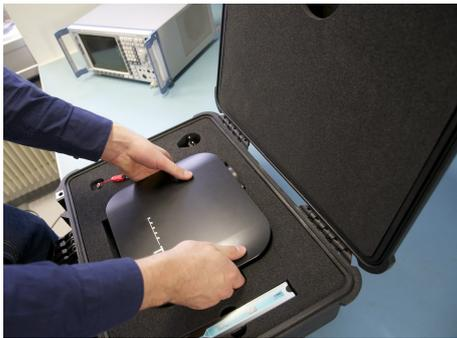
Remove the remote unit from the transport case as shown on the left.
