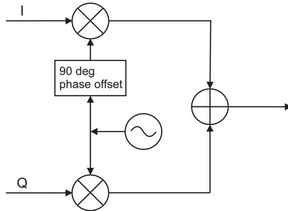
Figure 6.1: Block diagram of a quadrature modulator
