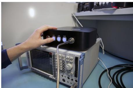
To activate the *RFoF1P* system on the desired channel press the corresponding button on the front side of the *Remote Unit*. Pressing the button for  $<0.5$  s will activate the channel for the measurement time programmed (see Chapter 5). Pressing the button for  $>0.5$  s will activate the channel permanently (the 0.5 s transition is visualized by a short "off-cycle" of the channel's LED).
