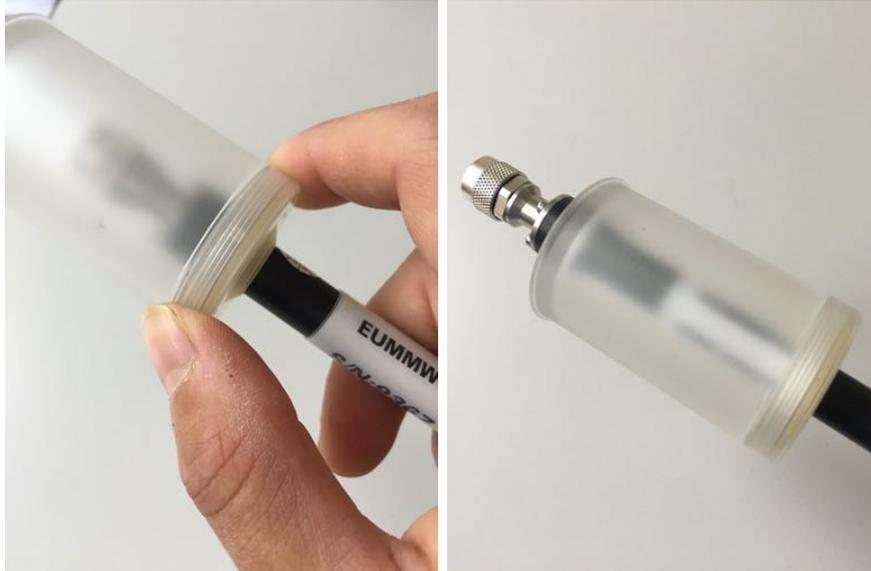
Align the notch and pin of the probe and DAE4ICEy connectors and carefully mate the probe connector with the DAE4ICEy connector. Make sure the probe body is straight and fasten the retainer nut carefully (not too tight). In the end screw on the probe cup and make sure the rubber seam is uniformly pointing upwards around the probe. Remove the protective cover before putting the probe inside the ICEy probe repository.
