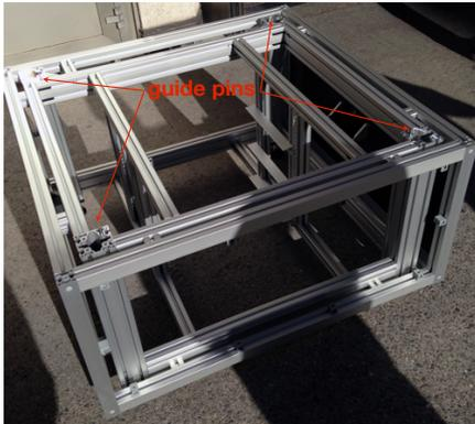
Locate the guide pins on the ICE $y$  Support. These pins will help to install the ICE $y$  test chamber, which has conical holes in its aluminium base, mating with the pins.
