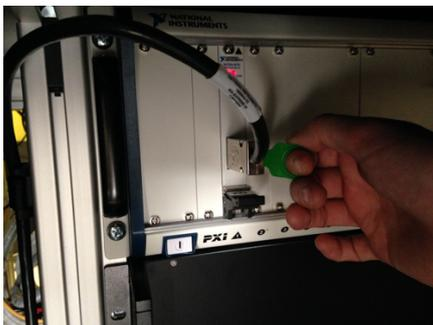
Fix the PXI inside the rack and connect the PXIe extension cable (from the Control PC) on the front side of the PXI chassis as shown.
