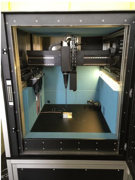
The ICE $y$  Test Chamber is located on top of the equipment rack. It is a fully RF shielded chamber with a door that opens to the right side. Inside the test chamber the positioning system which performs scanning is located. A LED light strip is located on the right side the probe repository holding up to 4 probes on the left side. Feedthroughs are available on the left and right sides as well as in the rear left corner.
