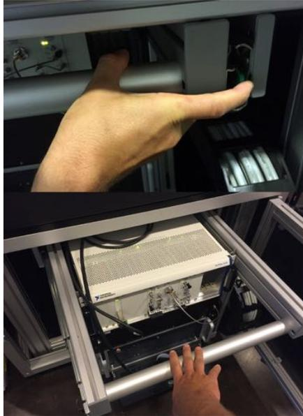
The 19 inch rack equipment is located in drawer for easier access for installation and maintenance. To move the equipment drawer out, fully open the front door, unlock the drawer by lifting the green lever (see photograph) and pull on the drawer handle.
