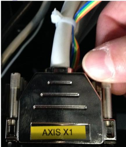
All connectors are individually labelled as shown on the left. Simply connect the connectors of all cables attached to the left side of the DIN rail on the rear side of the ICEy Support to the Test Chamber terminal according to the connector diagram shown in Figure 4.2
