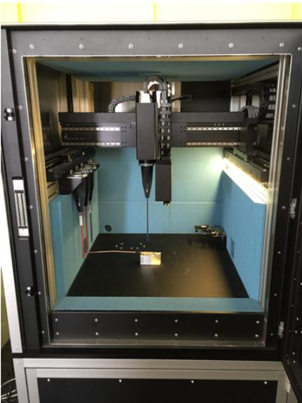
The camera system is suspended on the z-axis of the positioning system. In this way the camera system can scan across the workbench improving the the resolution of the scanning and allows direct correlation to the probe position.
