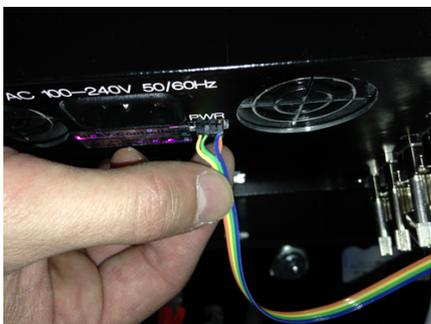
The IEICE $y$  power inhibit ribbon cable is connected using the small 8 pin power inhibit MOLEX 51110 connector on the rear-side of the IEICE $y$  close to the AC power inlet. Carefully, connect the small connector. When removing the connector, avoid pulling on the ribbon cable. The other end of the ribbon cable is connected inside the STANDBY/RST D-SUB cable connector, that should be connected to the IEICE $y$  before the MOLEX 51110.
