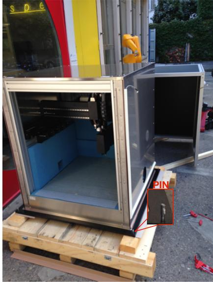
Lift the decorative housing (with 3 persons) sufficiently such that it is released from the locking pins shown on the left. Make sure not to lift the housing much further as it might otherwise not be possible to reverse with it. After lifting the housing from the locking pins, reverse with it and put it aside for later re-installation.
