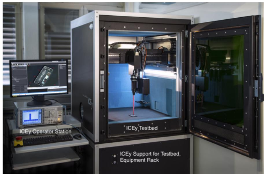
Figure 1.1: Interference and Compatibility Evaluation System (ICEy) setup. Shown is a typical system setup of ICEy with the system operator workplace on the left and the ICEy Test Chamber and the Support and Equipment Rack on the right.
