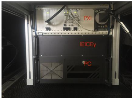
The ICEy rack drawer contain 3 19inch devices, the PXI Chassis with the Vector Signal Analyser, the IE-ICEy Interface Electronics and the Control PC.
