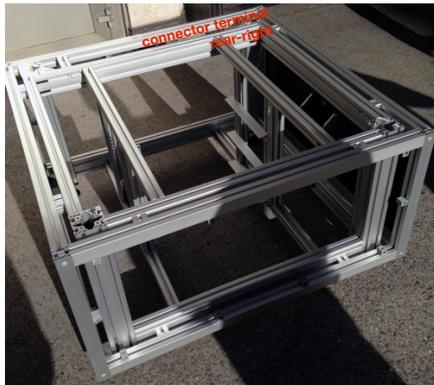
Remove the front and rear panels of the ICE $y$  Support as shown on the picture on the left. Place the Support on a flat surface such that the ICE $y$  Test Chamber can be mounted on top of it in the next step. **Ascertain that the feet are high enough to later get below the Support with the fork of a pallet jack.**
