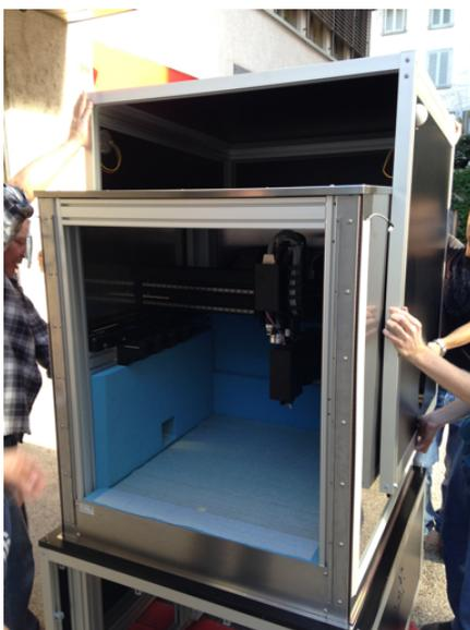
Now re-install the decorative housing as shown on the left. Also re-install the feed-through receptacle rings and close the JST connectors to the signal lamps and the door electronics again.
