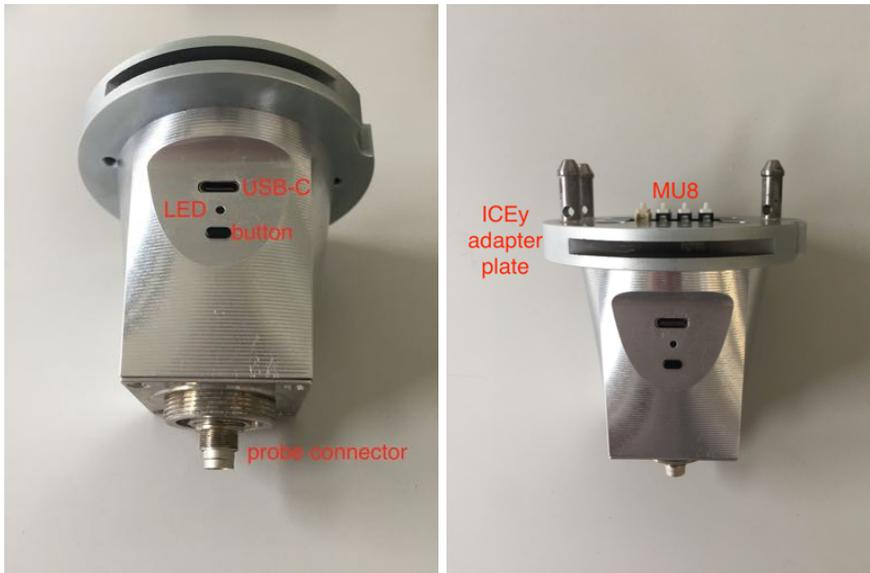
DAE4ICEy is a battery powered device and can be charged via the USB-C connector. Pressing the power button once will enable the DAE4ICEy and disable once pressed again. The LED will light up approximately 2s after activation and whenever the DAE4ICEy communicates with the TDS Remote Unit .
