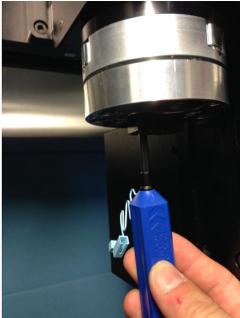
Clean the bottom (roll axis) MU8 adaptor using the click-cleaner (remove the blue cap again).
