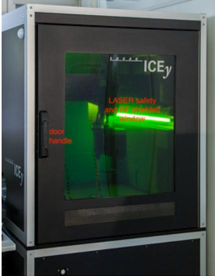
As mentioned above the door is equipped with an RF shielded window. In addition the door employs a (green) LASER safety window to attenuate the LASER radiation from the line LASERs. The chamber door is hinged on the right-hand side and can be opened using a handle on the left side.
