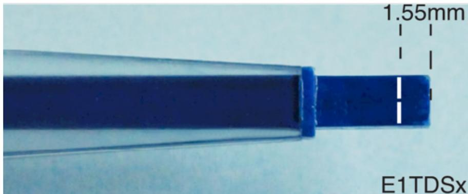
The dipoles of the E1TDS sensors are centred in the TDS probe tip centre. The tip to dipole centre distance is in both cases 1.55 mm.
