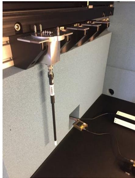
(b) The EUmmW probe positioned in slot 1 of the ICEy system.
