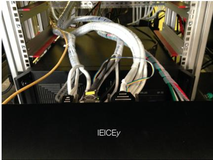
In the next step install the IEICE $y$  in the centre mounting rail of the rack. Again this 19" chassis can be wired from the front and then inserted as shown on the picture in the left.
