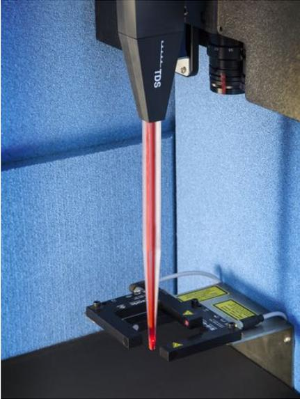
The probe tip location is reference in the fork light barriers. After *ICEy* picked up a probe its tip location is automatically referenced in the fork light barriers. During the reference also the repeatability of the light-barrier location is validated. The *ICEy* will warn the user if the repeatability is worse than 0.1 mm. A probe referencing can also be forced by the user from the *ICEy* GUI.
