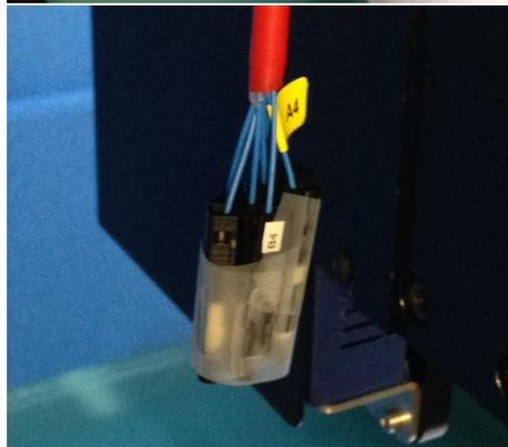
Prepare the new connector saver fiber optics by taping the 8 separate MU-simplex connectors together as shown. It is recommended not to remove the protective caps from the connectors.
