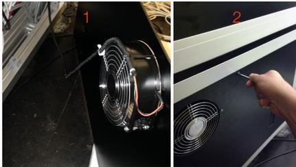
Place the rear panel inside the ICE $y$  Support frame (1). Make sure that the fan power cable is completely inside the system. Fix the rear-panel with the Allen screws provided from the outside (2).
