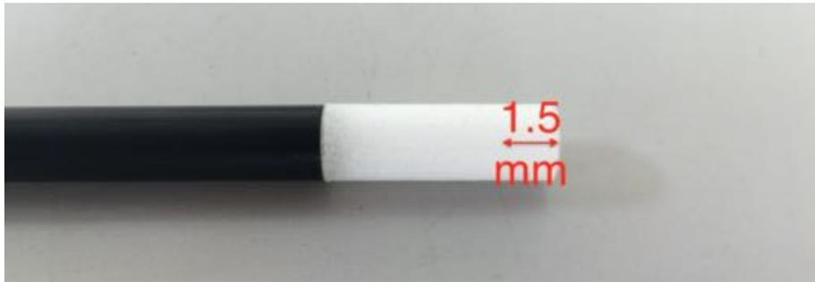
The sensors of the EUmmW probe are centred in the probe tip. The tip-to-sensor centre distance is 1.5 mm.
