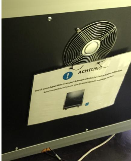
Like the test chamber, the rack has a fan providing ventilation to the equipment on the rear side. The fan is integrated inside the rear door and the fan speed is controlled by the rack temperature.
