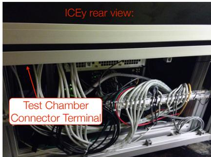
The ICEy Support is delivered pre-wired with all cables in place to connect to the connector terminal in this step as shown on the right.
