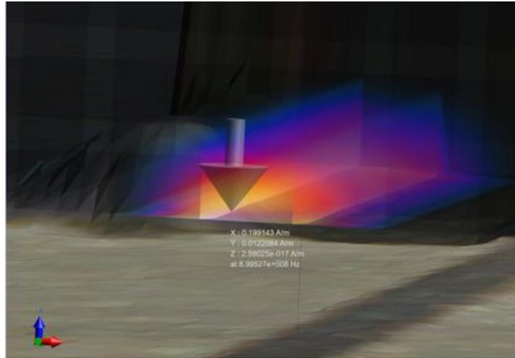
3. *Move to selected peak* : If ICEy is not in *Evaluator Only Mode*, a connected probe can be moved to the selected peak location (Figure 11.15).
