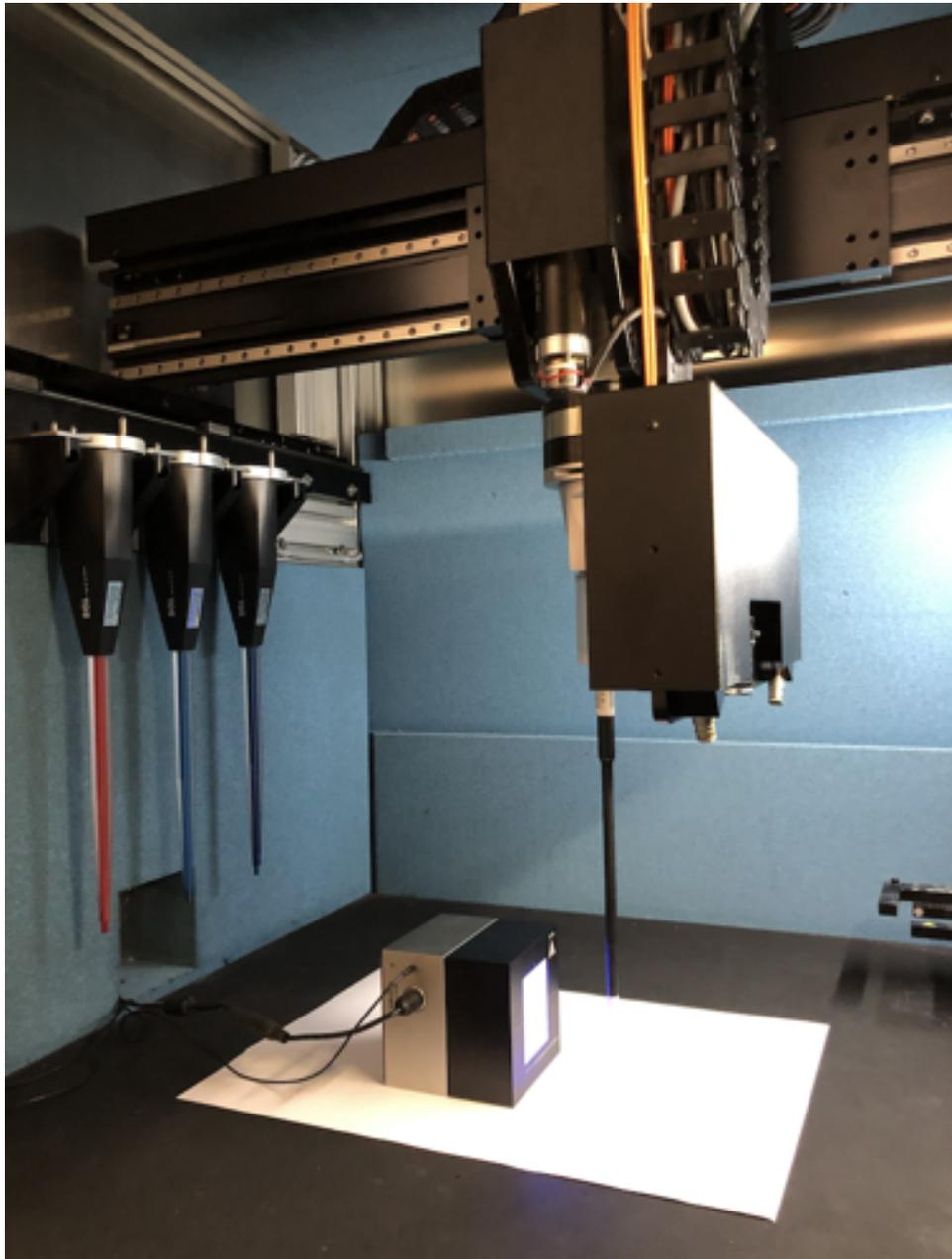
In this setup the verification source has been put on its side, radiating against the right side of the ICE $y$  test chamber. As the measurement plane will later be aligned in the x-z-plane of the system, we recommend to align the source parallel to the x-axis of the ICE $y$  system. It is also recommended to put a sheet of white paper below the source in order to differentiate it better in the camera scan from the black workbench floor.
