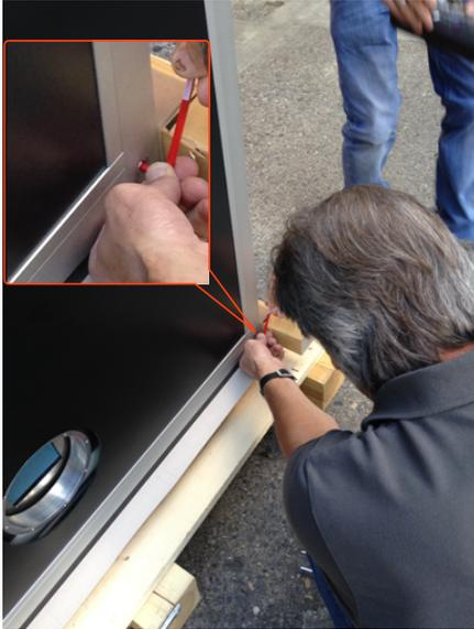
Remove the 4 grub screws at either corner of the decorative housing, securing it to the aluminium base of the ICEy Test Chamber as shown on the left using an Allen key.
