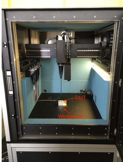
The ICE $y$  Test Chamber contains a platform made from laminated glass. This platform is called DUT Workbench. That is where the DUT can be placed. The glass platform has a thickness of 10 cm and is backed with an RF absorber.
