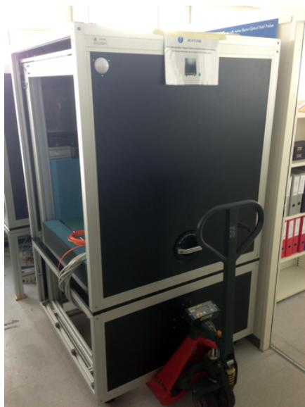
Use the pallet jack to move the entire ICEy to its destination. At the installation site use the adjustable feet to level the system and put it in place by lowering the pallet jack.
