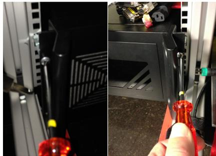
If the cable connectors had been mounted from the front side of ICEy slot the PC into the bottom most mounting rails of the rack and fix it using screws. Note: that the screws should go into 6 cm extenders. Also make sure that the rear mounting rails are positioned correctly before inserting the PC.
