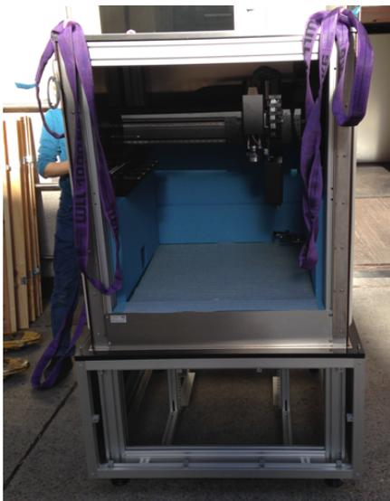
Use the crane or fork-lift to position the Test Chamber over the ICE $y$  Support. Slowly, lower the Test Chamber onto the Support and manually guide the Chamber into the guide pins.
