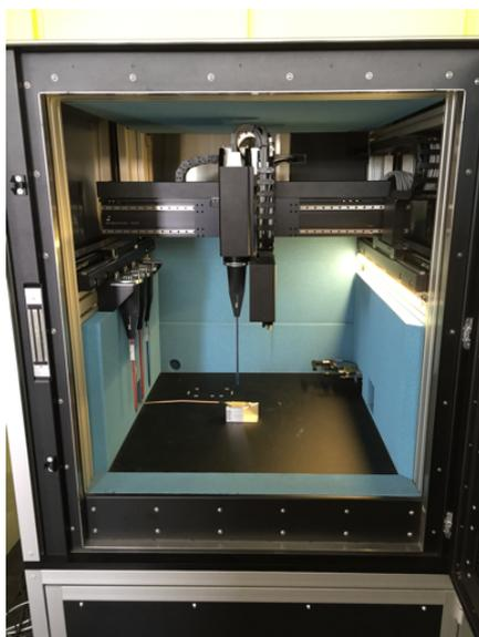
The ICEy Test Chamber can be illuminated by a LED light strip on the right hand side. As soon as the GUI starts up, the light is switched on. The light is switched off when the user exits the GUI. The light is also switched off during LASER scans.
