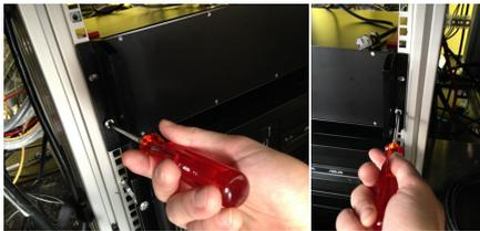
Secure the IEICE $y$  with screws inside the rack as shown on the left.
