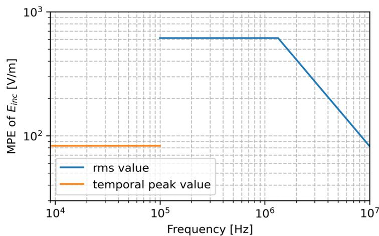
Figure 1.1: MPE limits of the incident E-field defined by the FCC. Note that the limits at frequencies  $\geq 100 \text{ kHz}$  are defined in terms of the *rms* value, while those at  $< 100 \text{ kHz}$  are defined in terms of the temporal peak value.
