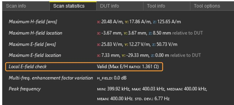
Figure 1.5: The section of the DASY8/6 Module WPT GUI that displays the statistical information of the volume scan, e.g., the result of the local E-field check (highlighted by the orange box; the maximum E/H ratio is also listed).
