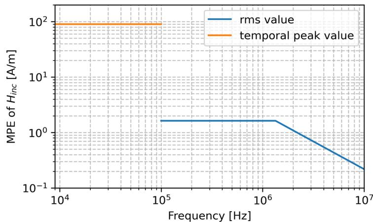
Figure 1.2: MPE limits of the incident H-field defined by the FCC. Note that the limits at frequencies  $\geq 100$  kHz are defined in terms of the *rms* value, while those at  $< 100$  kHz are defined in terms of the temporal peak value.
