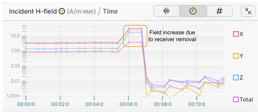
Figure 1.8: The time-domain plot of the incident H-field in the MAGPy graphical user interface. The data were recorded from a commercial wireless charger while removing the smartphone placed on the charger. The same procedure can also be used to monitor the stability of the source.
