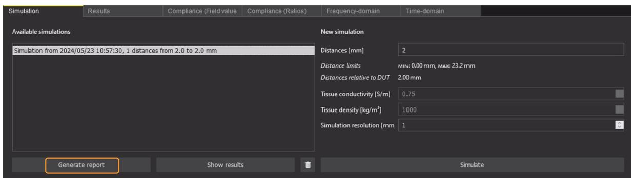
Figure 1.7: The section of the DASY8/6 Module WPT GUI for setting up the simulation and generating the report. Note that the tissue conductivity and mass density are pre-set to standardized values and cannot be altered by users. After the simulation is completed, a report can be generated by clicking the "Generate report" button (highlighted by the orange box).
