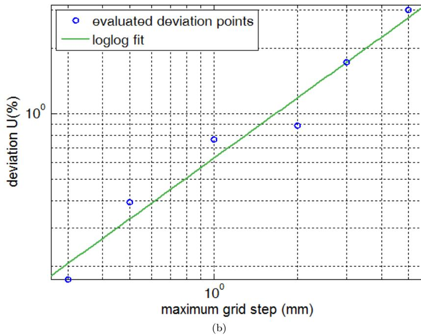
Figure 7: Maximum deviation (see equation (9)) of the numerical from the analytical solution along a circle at distance of 5mm (a), 10mm (b) 30mm (c) and 50mm (d) from the center of the sphere as a function of the maximum grid step.
