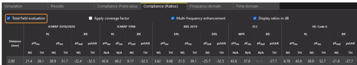
Figure 1.6: Table in the DASY8/6 Module WPT GUI showing the compliance evaluation results for the total induced SAR (i.e., for exposures from both incident H- and E-fields; note that the "Total field evaluation" option (highlighted by the orange box) is checked here). Since the coverage factor for 1 gram averaged SAR is one, there is no need to enable the coverage factor option.
