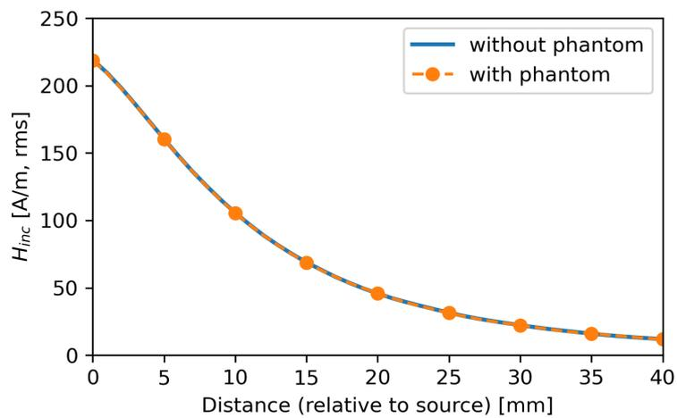
Figure 12: Comparison of the total incident H-fields (per  $1A_{\text{peak}}$ ) along the z-axis center line of the coil with and without the phantom for the reference source V-Coil 50/400.
