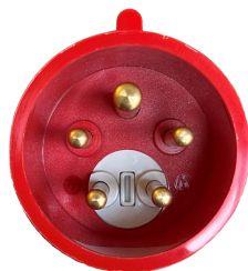
Figure 1.3: A 16A, 6h, 3P + N + G CEE connector
