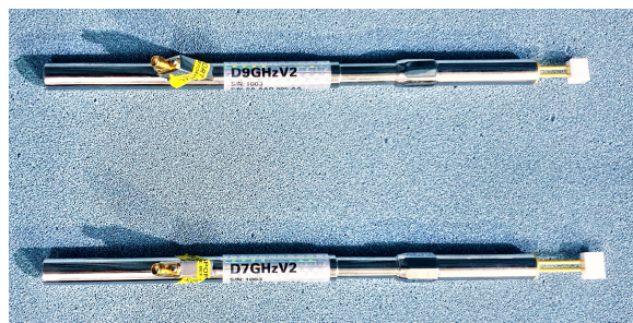
Figure 1.1: Two of the four dipoles (i.e., D7GHzV2 and the D9GHzV2) used for system performance checks in the frequency range between 6 – 10 GHz
