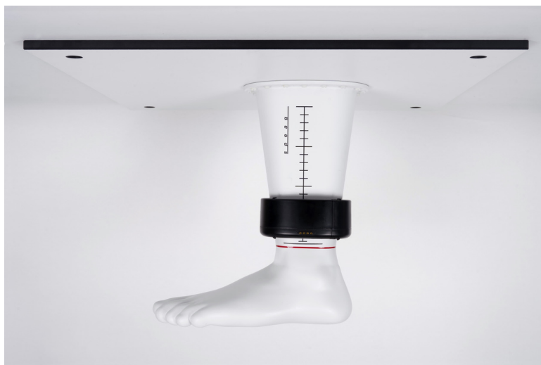
Figure 1.12: Electronic tag positioned on the Ankle Phantom aligned via the built-in ruler.
