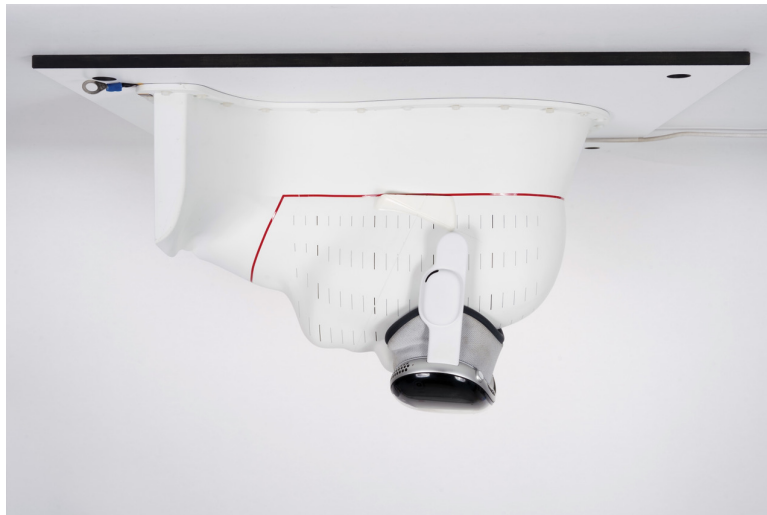
Figure 1.9: Smart goggles positioned on the Face-Down phantom; positioning lines ensure reproducible placement.
