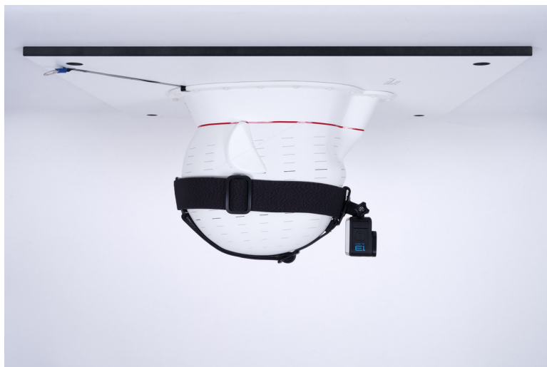
Figure 1.10: Smart camera positioned on the Head-Stand phantom; positioning lines ensure reproducible placement.
