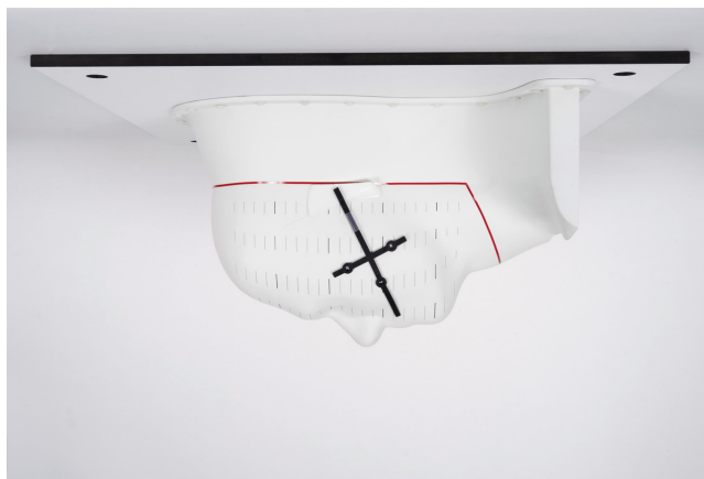
Figure 1.13: Facedown phantom with the mask mounted for accurate dipole positioning.
