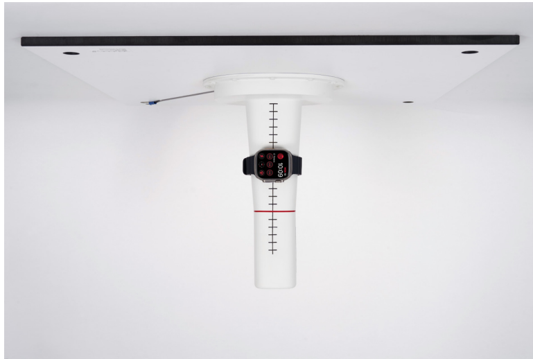
Figure 1.11: Smartwatch positioned on the Wrist Phantom aligned via the built-in ruler.
