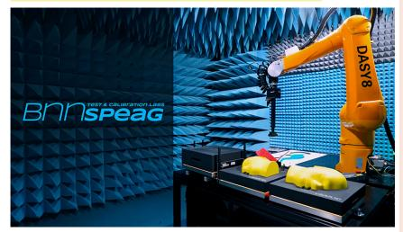
The promotional video of <u>BNNSPEAG</u> in New Delhi nicely illustrates how the latest DASY8<sup>3D</sup> system can be effectively used to evaluate all aspects of the most complex mobile devices, including specific absorption rate (SAR), mmWave (induced and absorbed power density (IPD/APD)), and WPT, covering the frequency range from 3 kHz to 110 GHz.
