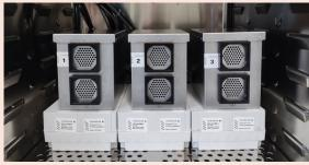
All three IT'IS exposure systems for controlled *in vitro*, animal, and human studies are now in operation at the laboratories of our <u>SEAWave</u> partners. The systems were developed, manufactured, and validated for use in risk assessments of 5th generation (5G) mobile communication systems (27.5 GHz).
