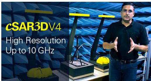
cSAR3D V4.0 marks another milestone for vector measurement-based systems. The new X10 Combiner eliminates the limitations previously posed by the fixed array and enables the frequency extension to 10 GHz. At the same time, it reduces the maximum deviations to less than 30%, even for very sharp SAR distributions. The new X10 Combiner is really simple to use, and no additional hardware is required. More detailed information, including a user video, can be found on our [website](#).
