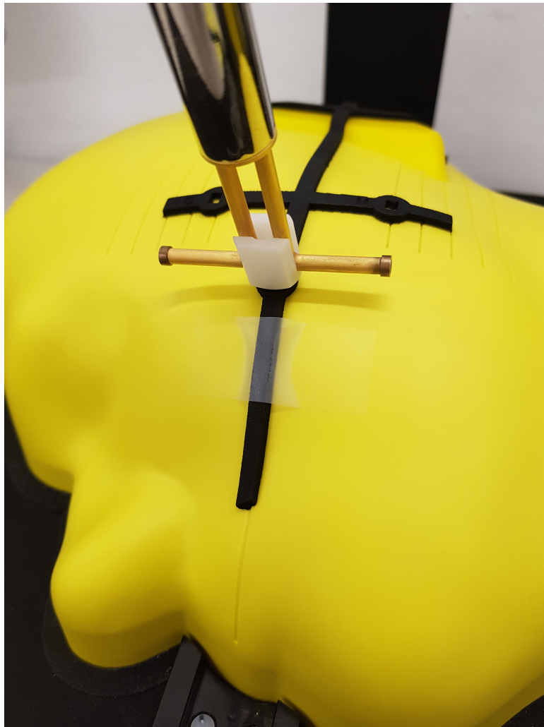
Figure 1.12: At the measurement location, the dipole shall be oriented so that a) the dipole arms are parallel to the phantom, b) the coaxial feed line is normal to the phantom, and c) the dipole arms are oriented at the correct angle.
