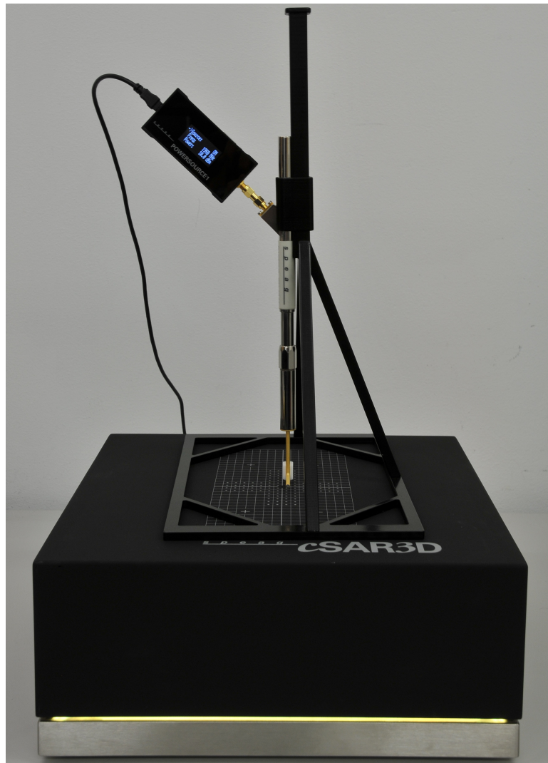
Figure 1.3: POWERSOURCE1 connected to validation dipole antenna for cSAR3D measurement.
