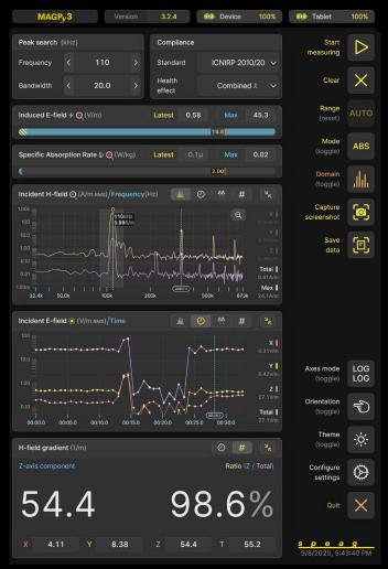
MAGPy3 GUI during an example measurement. Compliance with both RL and BR, shown as exposure ratios, are continuously updated during the measurement.
