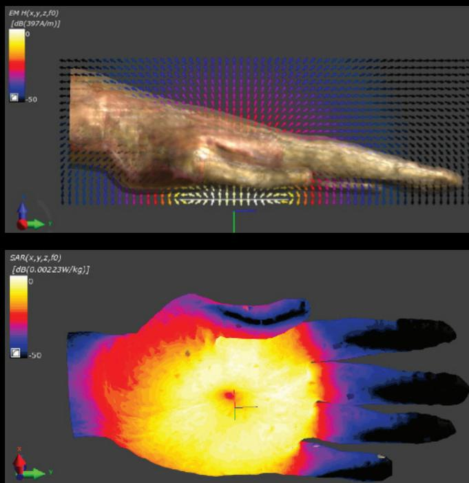
Example of the advanced evaluations: (top) reconstructed vector potential  $A$  of the imported measured H-field, (bottom) SAR distribution at the surface of the hand for the intended use case of picking up a mobile phone from a WPT charging station
